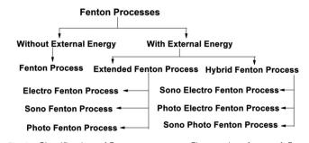
Fig. 1 Classification of Fenton processes. Figure taken from ref. 5.
