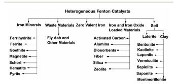
Fig. 2 Classification of heterogeneous Fenton catalysts.
