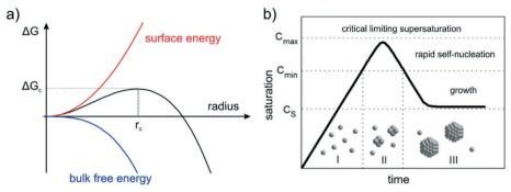
Fig. 1 (a) The dependence of the cluster free energy,  $\Delta G$ , on the cluster radius, r according to the classical nucleation theory (CNT). The curve has a maximum free energy  $\Delta G$  at a critical cluster size,  $r_c$ , which defines the first stable particles – the nuclei. (b) The principle of NP nucleation due to LaMer's mechanism of (sulfur) nucleation derived from CNT. The (theoretical) qualitative curve describes the monomer concentration as a function of time
