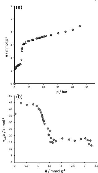
Fig. 2 Adsorption of CO<sub>2</sub> on MIL-53(Fe) at 303 K. (a) Isotherm repeated 5 times. (b) Enthalpies measured by calorimetry.
