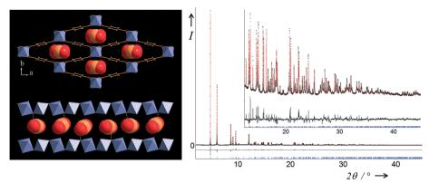
Fig. 5 Two views of the structure of MIL-53(Fe)[0.63CO<sub>2</sub>] (top left) in the ab plane showing stacked CO<sub>2</sub> molecules within all the lozenge-shaped channels and (bottom left) view of a single channel in the almost perpendicular direction. Final Rietveld plot (right) for MIL-53(Fe)[0.63CO<sub>2</sub>] from X-ray powder diffraction data measured at RT and 10 bar. Legend as Fig. 4.
