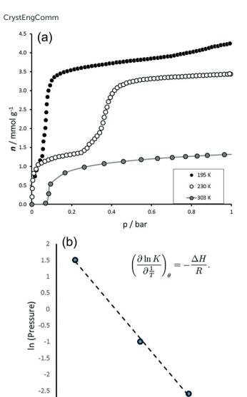
Fig. 1 Adsorption of CO<sub>2</sub> on MIL-53(Fe) to 1 bar. (a) Isotherms to 1 bar at 195 K, 230 K and 303 K. (b) Van't Hoff plot.
