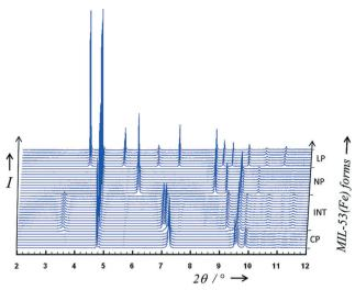
Fig. 3 Adsorption of CO<sub>2</sub> on MIL-53(Fe) followed by X-ray powder diffraction. Four different phases can be identified depending on the pressure and/or temperature (anhydrous CP, INT, NP and LP forms).
