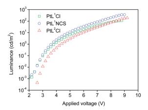
Fig. 7 Luminance versus applied voltage of the OLEDs using the neat complexes as emitting layers. The device incorporating PtL1Cl is shown in green, PtL<sup>1</sup>NCS is in blue, and PtL<sup>2</sup>Cl in red.
