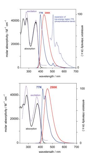
Fig. 1 Absorption (black), excitation (dashed purple), and emission (red lines) spectra of HL<sup>1</sup> (top) and HL<sup>2</sup> (bottom) in CH<sub>2</sub>Cl<sub>2</sub> at 298 K and their emission spectra at 77 K in diethyl ether-isopentane-ethanol (2:2:1 v/v) (blue lines).
