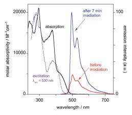
Fig. 4 Emission spectra of PtL<sup>2</sup>Cl in  $CH_2Cl_2$  at 298 K before and after irradiation with a UV lamp for 7 minutes ( $\lambda_{ex}=415$  nm).
