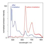
Fig. 5 Emission spectra of  $PtL^2Cl$  at 77 K in diethyl ether—isopentane—ethanol (2 : 2 : 1 v/v) before and after UV irradiation.
