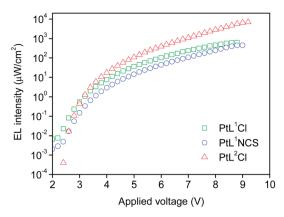
Fig. 8 Electroluminescence intensity versus applied voltage of the OLEDs using the neat complex as EML; colours as in Fig. 7.
