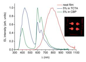
Fig. 10 Electroluminescence spectra of OLEDs incorporating PtL<sup>2</sup>Cl as a neat film or doped in TCTA or CBP as the emitting layer at 8 V. Photo of the NIR-OLEDs (inset)
