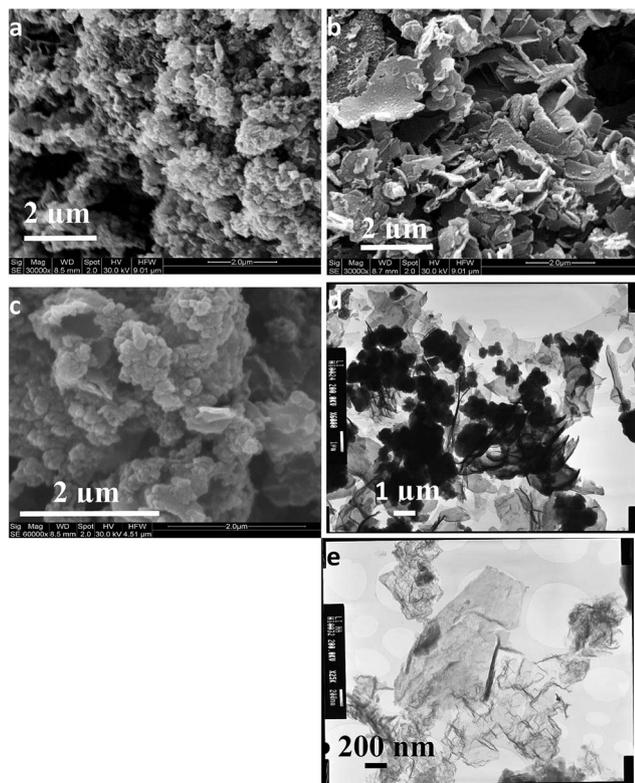
Fig. 4 SEM and TEM images of carbon deposited at 4 V in (a and b)  $\text{Li}_2\text{CO}_3\text{-Na}_2\text{CO}_3$  at 550 and 700 °C respectively, (c)  $\text{Li}_2\text{CO}_3\text{-K}_2\text{CO}_3$  at 700 °C, (d)  $\text{Li}_2\text{CO}_3$  at 722 °C and (e)  $\text{Li}_2\text{CO}_3\text{-Na}_2\text{CO}_3$  at 700 °C; atmosphere:  $\text{CO}_2$ .
