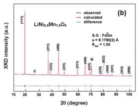
Fig. 3 (a) XRD patterns of the spinel samples at different steps of the synthesis in the temperatures range 700–900 °C before annealing, and for the final sample, post-annealed at 600 °C for 48 h. Inset shows the magnified Bragg lines between  $2\theta=35-45^\circ$  with impurity peaks marked by arrows (b) Rietveld refinement profiles of the XRD data for the LNM electrode film (Si peak comes from sample holder). Reproduced with permission.  $^{64}$
