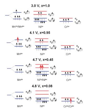
Fig. 9 Schematic diagram showing the 3d electronic levels of  $Mn^{3+}$ ,  $Ni^{2+}$  and  $Cr^{3+}$  in  $LiNi_{0.5-y}Mn_{1.5-y}Cr_{2y}O_4$  spinel during the charge process. It is noted that  $Ni^{2+}$  favours the low-spin configuration in  $LiNi_{0.5-y}Mn_{1.5-y}Cr_{2y}O_4$ . Partially empty levels are shown with red arrows.
