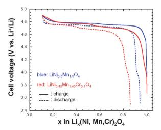
Fig. 10 Charge–discharge curves of the un-doped and Cr-doped LNM cathodes in CR2032 coin cell composed of LiPF $_6$  in EC–DEC (1 : 1) as electrolyte. The cathode electrode contained 89 wt% active material, 6 wt% conductive carbon, and 5 wt% PVdF binder (loading 5 mg cm $^{-2}$ ). All cells were cycled at 25 °C between 3.5 and 4.9 V at C/5 rate.
