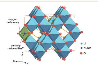
Fig. 1 The structure of spinel  $LiNi_{0.5}Mn_{1.5}O_4$  ( $Fd\bar{3}m$  S.G.). Oxygen deficiency partially reduces Mn<sup>4+</sup> to Mn<sup>3+</sup> to satisfy local charge neutrality.
