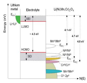
Fig. 7 Schematic density of states and Fermi energies for  $\text{Li}_x \text{Ni}_{0.5-y^-}$  Mn<sub>15-y</sub>Cr<sub>2y</sub>O<sub>4</sub> spinel cathode. The Li permeable SEI layer formed on the electrode surface preserves the overall reversible reaction.
