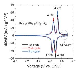
Fig. 11 Differential capacity curves, dQ/dV vs. V, of the un-doped LNM (top) and LiNi<sub>0.45</sub>Mn<sub>1.45</sub>Cr<sub>0.1</sub>O<sub>4</sub> (bottom). The values at the peaks are given in volt. Reproduced with permission.<sup>64</sup>
