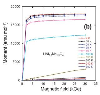
Fig. 6 (a) Inverse of the magnetic susceptibility H/M measured at H=10 kOe, for the  $\text{LiNi}_{0.45}\text{Mn}_{1.45}\text{Cr}_{0.1}\text{O}_4$  samples after post annealing at 600 °C and the  $\text{LiNi}_{0.45}\text{Mn}_{1.45}\text{Cr}_{0.1}\text{O}_4$  crystallized in the same  $Fd\overline{3}m$  space group. (b) Magnetization curves of the  $\text{LiNi}_{0.5}\text{Mn}_{1.5}\text{O}_4$  sample crystallized in the  $Fd\overline{3}m$  space group. Reproduced with permission.<sup>64</sup>
