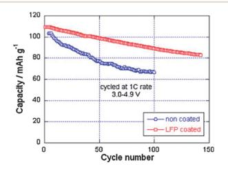
Fig. 17 Cyclability of the Li//LMN and Li//LFP-coated LMN cells at 1 C between 3.0 and 4.9 V vs.  $\rm Li^+/Li^0$ . Reproduced with permission.<sup>86</sup>
