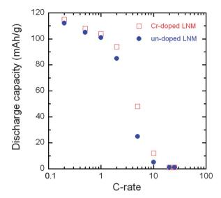
Fig. 12 Modified Peukert curves of LNM and LiNi $_{0.45}$ Mn $_{1.45}$ Cr $_{0.1}$ O $_4$  spinel cathodes cycled between 3.5 and 4.9 V in CR2032 coin cell with LiPF $_6$  in EC-DEC (1 : 1) as electrolyte.
