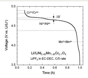
Fig. 8 Typical voltage profile of charge of a Li//Cr-doped LNM cell showing the various redox reactions  $\rm Mn^{3+/4+}$  (at 4.1 V),  $\rm Ni^{2+/4+}$  (at 4.7 V) and  $\rm Cr^{3+/4+}$  (at 4.8 V).
