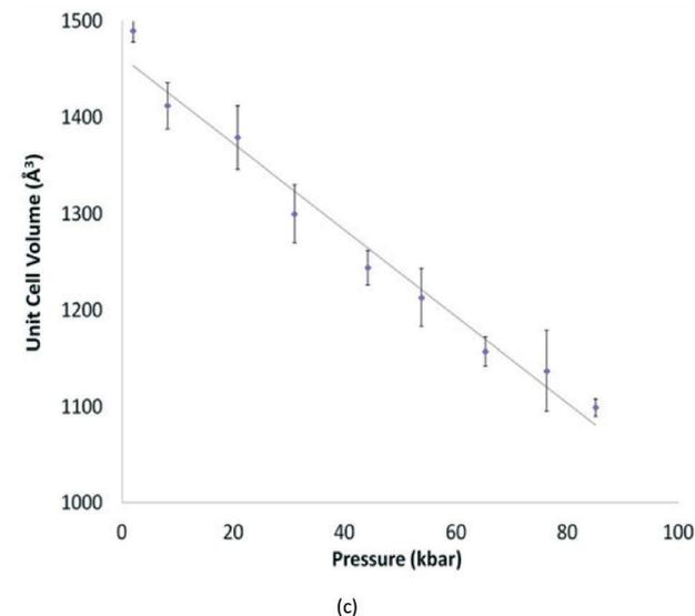
Fig. 4 Unit cell volume ( $\text{\AA}^3$ ) vs. pressure (kbar) for 1 (a, blue), 2 (b, red) and 3 (c, purple). Error bars indicate  $3\sigma$  limits. Pressure values are an average of measurements taken before and after the data collection. The solid line is a guide to the eye.
