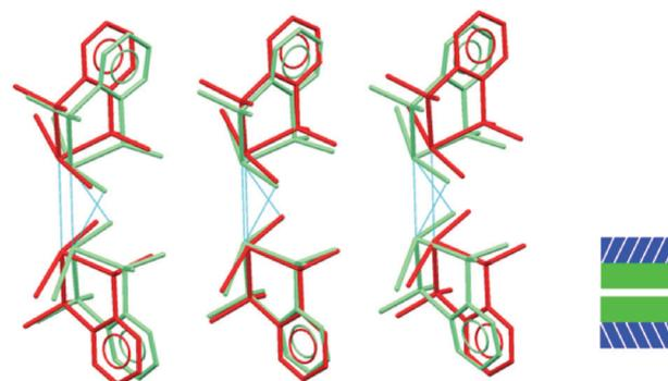
Fig. 7 Showing superposition of low pressure (red) and high pressure (green) forms of 2 illustrating that the  $\text{GeBr}_2\cdots\text{Br}_2\text{Ge}$  interlayer separation decreases, but does not otherwise change.
