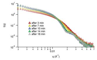
SAXS profiles for the *in situ* micelle-to-vesicle transition.
