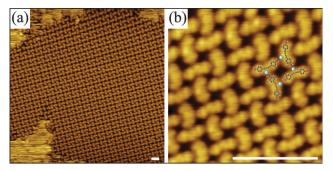
Fig. 3 (a, b) Ordered phase of  $\bf 1$  on Cu(001). Molecules were deposited at 300 K and subsequently annealed at 450 K for 5 min. (b) Blue spheres indicate some Cu adatoms. Images acquired at 300 K. Scale bars are 5 nm.
