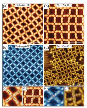
Fig. 1 (a) Fe-1 and (b) Ni-1 fully reticulated network structures on Au(111) (metal atom: 1 ratio 1:1). The same Fe-1 networks can also be obtained on (c) Ag(001) and (d) Cu(001) substrates. Models for each structure are shown in the corresponding bottom panels. Structures were obtained by simultaneous deposition of metal atoms and 1 at 450 K on the substrates. Images acquired at 5 K (a, b) and 300 K (c, d). Scale bars are 5 nm.
