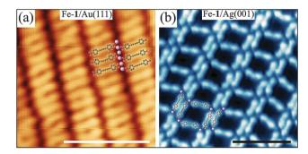
Fig. 2 (a) Fe-rich row phase on Au(111). Fe:1 ratio 2:1. (b) Fe-deficient double-row structure on Ag(001). Fe:1 ratio: 2:3. Structures were obtained by simultaneous deposition of Fe and 1 at 450 K. Images acquired at 5 K. Scale bars are 5 nm.
