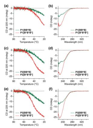
Fig. 3 CD cooling curves (a, c and e) and spectra at 20 °C (b, d and f) for **Pn[BB\*B]** (green) and **Pn[B\*B\*B\*]** (red) (n = 1,2, and 3;  $c_{BTA} = 50 \mu M$  in DCE; cooling rate:  $1 \,^{\circ}$ C min<sup>-1</sup>). (a, b) **P1** (c, d) **P2**, and (e, f) **P3** series of polymers.
