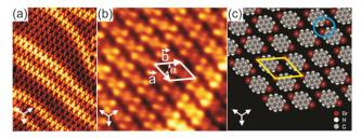
Fig. 2 (a) Overview STM image  $(24 \times 15 \text{ nm}^2)$  for 1 ML of Br<sub>2</sub>Py on Au(111). (b) Close-up STM image  $(6.5 \times 6.5 \text{ nm}^2)$  and (c) corresponding proposed molecular model. The STM images were taken at 77 K with U = -1.8 V, I = 30 pA.
