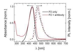
**Fig. 9** Normalised absorbance (solid lines) and PL (dashed lines) spectra of the aqueous solution of **P2** (0.01 g  $L^{-1}$ ) in the presence and absence of 0.17 μM of antibody at 20 °C. The absolute PL spectra are given in Fig. S10.†
