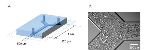
Fig. 1 Microfluidic device for defined engineering of vascular structures. A. Schematic overview of the polydimethylsiloxane–glass device showing the dimensions and geometry of the microchannel. B. Bright field micrograph of the cell suspension inside the microchannel, one hour after seeding
