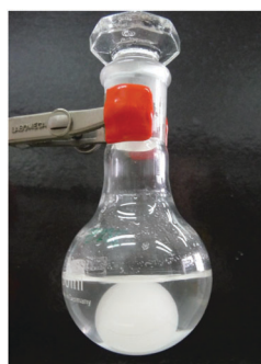
Fig. 1 Separation of [PBu_4][NTf_2] (paraffin ball) from water layer in ILICM process.
