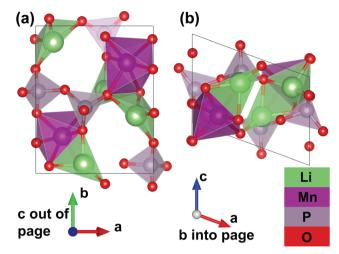
Fig. 3 The unit cell structure of the fully discharged  $\gamma$ -Li<sub>2</sub>MnP<sub>2</sub>O<sub>7</sub>. (a) Shows the c-axis, the tunnel direction, pointing into and out of page, and (b) shows the c-axis pointing up and down. This structure is in the  $P2_1$ spacegroup (a = 7.27 Å, b = 8.55 Å, c = 5.12 Å, and  $\alpha$  = 90°,  $\beta$  = 110°,  $\gamma$  = 90°). Identifier from the materials project: mp-770967.
