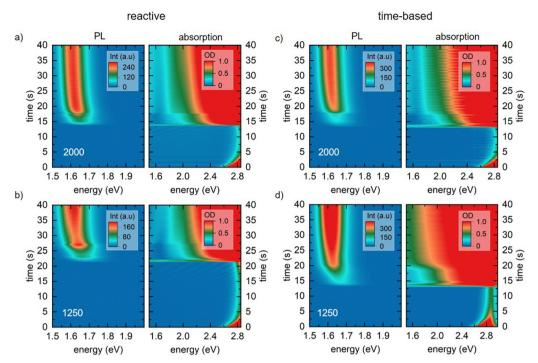
Fig. 3 Heat maps of photoluminescence (left) and absorption (right) measurements of MAPbI<sub>3</sub> solutions during spin coating via the reactive spin coating approach (a) and (b) and for the time-based approach (c) and (d) for spin speeds of 2000 and 1250 rpm.
