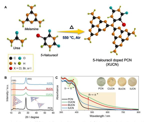
Fig. 1 Structure and optical properties. (A) Schematic illustration of the preparation of a 5-halouracil doped polymeric carbon nitride catalyst (XUCN), (B) powder X-ray diffraction (XRD) profiles, and (C) UV-visible diffuse reflectance spectra (UV-vis DRS) with digital photographs of powder catalyst as inset.
