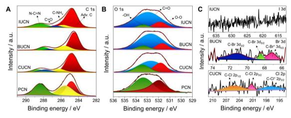
Fig. 2 Deconvoluted high-resolution X-ray photoelectron spectrum for (A) C 1s, (B) O 1s, and (C) Cl 2p, Br 3d, and I 3d of PCN and XUCN (X = Cl, Br, or I) samples.
