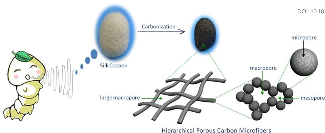
Figure 4: Pictorial representation of preparation of hierarchical porous CMF from silk cocoon. Reproduced with permission from [30] Copyright (2013) Nature Scientific Reports.
