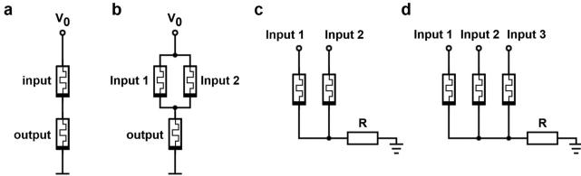
Fig. 3 Schematic of the memristor-based (a) NOT gate, (b) NOR gate, (c) IMP gate, and (d) NAND gate. (a) and (b) Reproduced with permission. 141 Copyright 2017, Springer Nature. (c) and (d) Reproduced with permission.<sup>53</sup> Copyright 2021, Royal Society of Chemistry.
