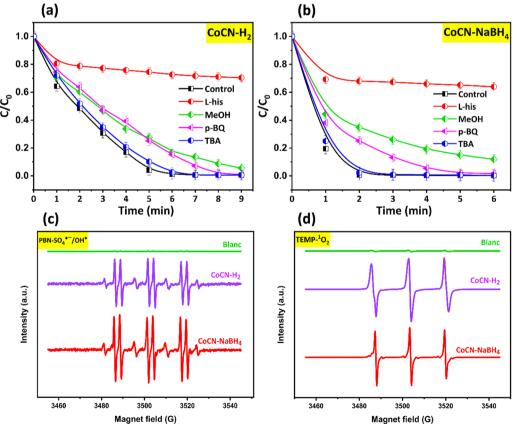
Fig. 10 Scavenger effect experiments on OG removal in (a) the CoCN $-H_2/PMS$  system, and (b) CoCN $-NaBH_4/PMS$  system, and EPR signals of different active free radicals (c) PBN $-SO_4^{\bullet-}/OH^{\bullet}$  and (d) TEMPO $^{-1}O_2$ .
