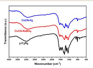
Fig. 4 FTIR spectra of CoCN-H<sub>2</sub>, CoCN-NaBH<sub>4</sub>, and g-C<sub>3</sub>N<sub>4</sub>.
