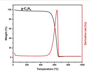
Fig. 1 TGA curve of g-C<sub>3</sub>N<sub>4</sub>.
