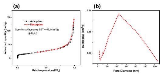
Fig. 7 BET isotherms (a) and pore-size distribution curve (b) of the g-C<sub>3</sub>N<sub>4</sub> support.
