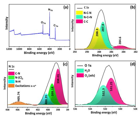
Fig. 2 (a) XPS survey spectrum, and high resolution XPS spectra of (b) C 1s, (c) N 1s, and (d) O 1s of  $q-C_3N_4$
