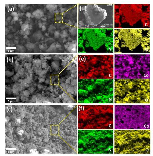
Fig. 5 SEM micrographs and EDS mapping of (a) and (d)  $g-C_3N_4$ , (b) and (e)  $CoCN-NaBH_4$ , and (c) and (f)  $CoCN-H_2$ .
