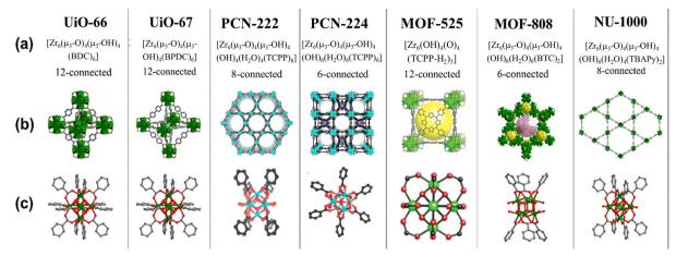
Scheme 2 Selected Zr-MOFs and their structures: (a) notations and formulations for the selected MOFs; (b) MOF structure; and (c) structures of the corresponding building units. Reproduced with permission from ref. 18,25,26. Copyright 2012, 2019 American Chemical Society.
