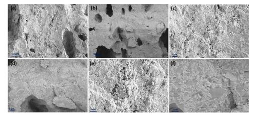
Fig. 12 Cross-sectional SEM images of (a), (c) and (e) 100-layers and (b), (d) and (f) drop-cast porous NLK-GDC symmetric cells in 1.23k× (a and b),  $3.71k\times$  (c and d), and  $9.77k\times$  (e and f) magnifications.
