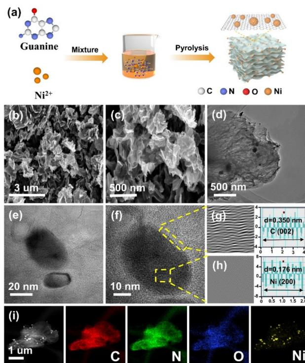
**Fig. 1** (a) Schematic illustration of the preparation of Ni@NC- $X$ . (b and c) SEM images of Ni@NC-1000. (d) TEM image of Ni@NC-1000. (e and f) HRTEM image of Ni@NC-1000. (g and h) FFT images and the corresponding interplanar spacing images of the square marked areas. (i) Elemental mapping images of C, N, O and Ni of Ni@NC-1000.
