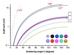
Fig. 4 Transferred energy  $E_{\rm T}$  against the elastic scattering angle  $\Theta$  for all studied elements. In red are the angles indicated, at which  $E_T$  exceeds  $E_d$ .
