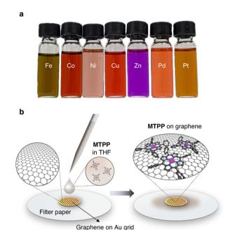
Fig. 2 TEM Sample preparation. (a) Image of the used 1.5 mM solutions of MTPPs in THF. (b) Illustration of the solution-based deposition of MTPPs on the graphene grid.
