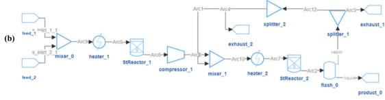
Fig. 14 Optimal flowsheets for methanol system with 18 units in pool. (a) product flow rate = 0.892 mol s<sup>-1</sup>, cost per mole product = 0.035 \$ per mol; (b) product flow rate =  $0.979 \text{ mol s}^{-1}$ , cost per mole product = 0.051\$ per mol.
