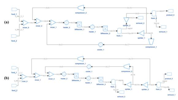
Fig. 11 Optimal flowsheets for HDA system with 20 units in pool. (a) product purity = 99.9%, product flow rate = 0.240 mol s<sup>-1</sup>; (b) product purity = 95.9%, product flow rate =  $0.288 \text{ mol s}^{-1}$
