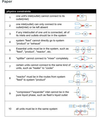
Fig. 3 Physics constraints energy or chemical systems must follow (H, R, C, F, O in the plot denote heater, reactor, compressor, flash drum and any other unit)
