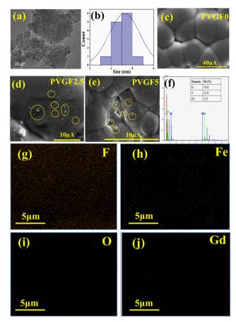
Fig. 2 (a) and (b) TEM image and the size distribution curve of Gdincorporated  $\alpha$ -hematite. (c)–(e) FESEM micrographs of PVGF0, PVGF2.5, PVGF5. (f) EDX images Gd-incorporated hematite NPs. (g)-(j) Mapping of the PVGF2.5 membrane suggesting the homogeneous distribution of doped-Gd-incorporated hematite in the PVDF matrix. The carbon distribution of the membrane is not shown due to the use of carbon tape during the EDS mapping measurement.
