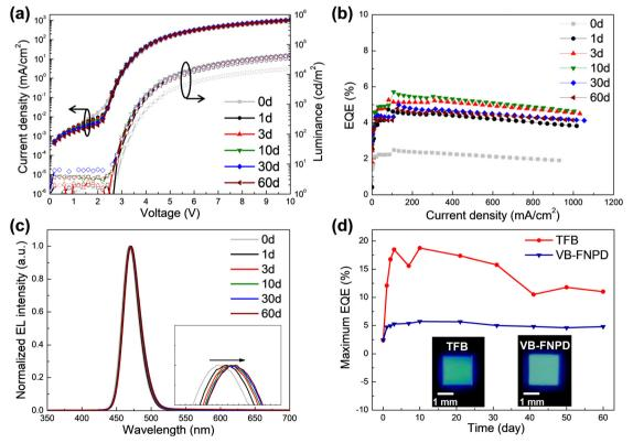
Fig. 4 (a) J-V-L, (b) EQE-J, and (c) EL spectra of encapsulated B-QLEDs with VB-FNPD as HTL stored for different days in a nitrogen-filled glovebox. (d) EQE<sub>max</sub> of B-QLEDs with different HTL changes with time. Insets are the encapsulated B-QLEDs with TFB and VB-FNPD as HTL stored for 60 days in a nitrogen-filled glovebox.
