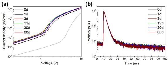
Fig. 2 (a) J-V curves of the encapsulated electron-only devices with structure ITO/ZnO sol-gel/B-QDs/ZnMgO/Al stored for different days in a nitrogen-filled glovebox. (b) TRPL decay curves of glass/B-QDs/ZnMgO/Al with encapsulation stored for different days in a nitrogen-filled glovebox.
