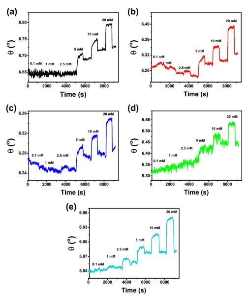
Fig. 3 Dynamic responses of M-BDC-functionalized SPR sensors towards different concentrations of glucose (0.1, 1, 2.5, 5, 10, and 20 mmol L<sup>-1</sup> in PBS solution): (a) bare Au substrate, (b) Cu-BDC, (c) Ni-BDC, (d) Mn-BDC, and (e) Zr-BDC
