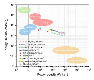
Ragone plot of Ni(OH)<sub>2</sub>//AC hybrid supercapacitors.<sup>46–51</sup>
