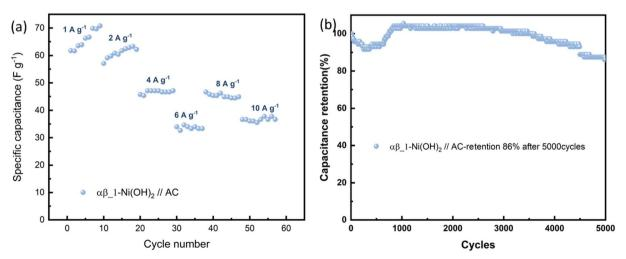
Fig. 11 (a) The specific capacitance evolution under various current densities of  $\alpha\beta_1$ -Ni(OH)<sub>2</sub>//AC. (b) Cycling performance at 100 mA cm<sup>-1</sup> for 5000 cycles.
