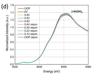
Fig. 9 In situ Ni K-edge XANES spectra of (a)  $\alpha$ -Ni(OH)<sub>2</sub>, (b)  $\alpha\beta$ \_1-Ni(OH)<sub>2</sub>, (c)  $\alpha\beta$ \_2-Ni(OH)<sub>2</sub> and (d)  $\beta$ -Ni(OH)<sub>2</sub> under a oxidation and reduction scans.
