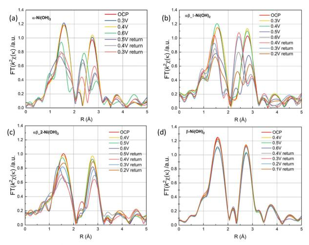
Fig. 10 The FT signal of the  $\kappa^2$ -weighted EXAFS (a)  $\alpha$ -Ni(OH)<sub>2</sub>, (b)  $\alpha\beta$ \_1-Ni(OH)<sub>2</sub>, (c)  $\alpha\beta$ \_2-Ni(OH)<sub>2</sub> and (d)  $\beta$ -Ni(OH)<sub>2</sub> under a oxidation and reduction scans.
