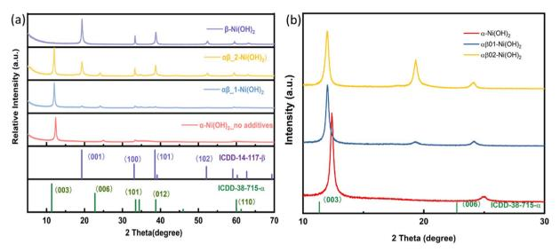
Fig. 1 (a) PXRD patterns of nickel hydroxide powder prepared with additive NH<sub>4</sub>F. (b) Expanded 2 theta region of PXRD patterns highlighting the 003 and 006 reflections of the alpha phase for  $\alpha$ -Ni(OH)<sub>2</sub>,  $\alpha\beta$ \_1-Ni(OH)<sub>2</sub>.
