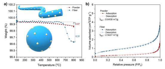
Fig. 4 Exsolution process of LCNT perovskite materials under chemical reduction. (a) Weight loss of LCNT samples reduced in  $5\% H_2/N_2$  from 100 to 800 °C, (b)  $N_2$  adsorption–desorption isotherms and BET surface area of samples.
