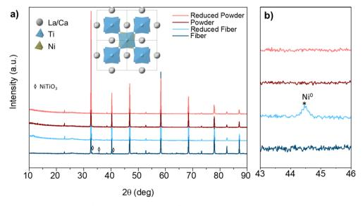
Fig. 1 Exsolution of Ni nanoparticles from LCNT perovskite materials. (a) XRD pattern of powder and fibers samples before and after reduced in  $5\% H_2/N_2$  at  $800 \, ^{\circ}$ C for 4 h. (b) The magnified  $2\theta$  range between 43 to  $46^{\circ}$  to illustrate the presence of Ni phase.
