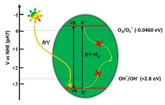
Fig. 21 Schematic of the photocatalytic process.
