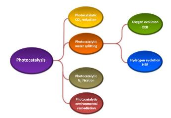
Fig. 11 Various reactions catalysed by g-C<sub>3</sub>N<sub>4</sub> based SACs in the area
