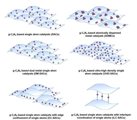
Fig. 1 Various configurations of metal atom dispersions over g-C<sub>3</sub>N<sub>4</sub> matrix.
