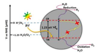
Fig. 15 Schematic diagram of photocatalytic water splitting.
