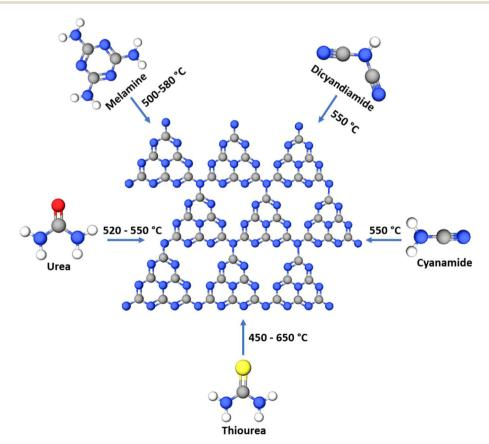
Fig. 4 Synthesis of g-C<sub>3</sub>N<sub>4</sub> from various nitrogen abundant precursors.
