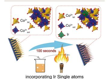
Fig. 13 Schematic illustration of synthesizing Ir SA incorporated Co<sub>3</sub>O<sub>4</sub> NWs. Copyright 2022, Wiley-VCH.
