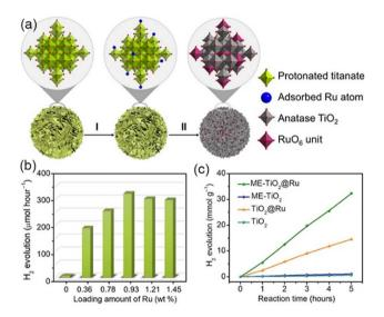
Fig. 4 (a) Illustration of the synthetic route to Ru SAs in TiO<sub>2</sub>. (b) Photocatalytic H<sub>2</sub> generation rates of ME-TiO<sub>2</sub>@Ru with different Ru loading amounts. (c) Time-dependent hydrogen evolution activities. Copyright 2020, the author, and American Association for the Advancement of Science
