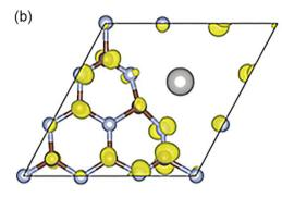
Fig. 2 (a) Energy-band alignment diagrams for  $g-C_3N_4$  and  $g-C_3N_4-Pt^{2+}$ . (b) Photoexcited charge density transition from the  $Pt^{2+}$ -induced hybrid highest occupied molecular orbital (HOMO) states to the lowest unoccupied molecular orbital (LUMO) of  $g-C_3N_4-Pt^{2+}$ . Copyright 2016, Wiley-VCH.
