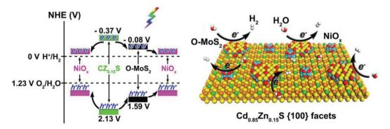
Fig. 10 Energy-band alignments of  $CZ_{0.15}S$ ,  $O-MoS_2$ , and  $NiO_x$  (left) and a schematic showing the photocatalytic hydrogen evolution over  $CZ_{0.15}S@O-MoS_2/NiO_x$  (right image). Copyright 2019, Wiley-VCH.
