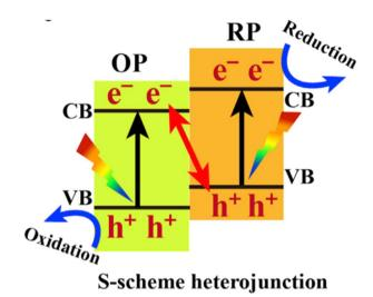
Fig. 11 Band structure configuration and charge-transfer route of the S-scheme heterojunction. Copyright 2020, Elsevier Inc.
