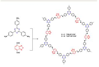
Fig. 17 Synthesis of TPB-BT-COF and TAPT-BT-COF.
