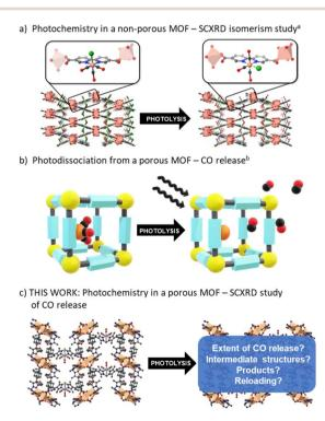
Fig. 1 Representations of (a) prior art interrogating the photochemistry of M(diimine)(CO) $_3$ X in a MOF (note the Cl $^-$  ligand shifts from an axial to equatorial site upon photolysis but is not quantitative and this leads to disorder) and (b) applying it to generate a MOF-based photoCORM. Herein, (c) we probe the chemistry of M(diimine)(CO) $_3$ X photolysis in a permanently porous MOF, providing crystallographic snapshots of the photolysis process.
