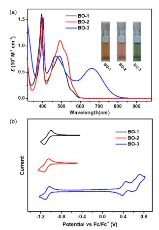
Fig. 3 (a) UV-vis-NIR absorption spectra of BO-1-3 in DCM ( $10^{-5}$  M). Inset: photo image of BO-1-3 in DCM solution. (b) Cyclic voltammogram of BO-1-3 (1.0 mM in DCM) with 0.10 M TBA-PF<sub>6</sub> as the supporting electrolyte.
