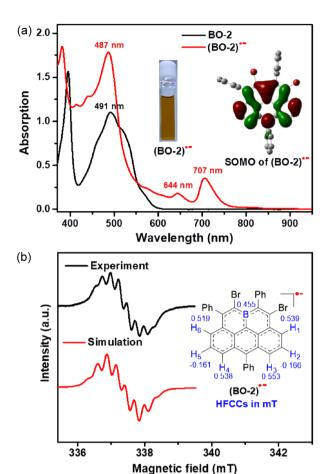
Fig. 4 (a) UV-vis-NIR absorption spectra of BO-2 and (BO-2)\* in DCM (10<sup>-5</sup> M). Inset: photo image of (BO-2)\* in DCM and DFT calculated SOMO distribution (UB3LYP/6-31G(d,p)). (b) Observed and simulated ESR spectra for (BO-2)\* in DCM at 293 K with hyperfine coupling constants (HFCCs).
