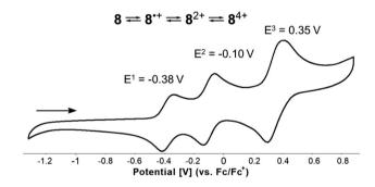
Fig. 9 Cyclic voltammogram of the N-doped molecular saddle 8.
