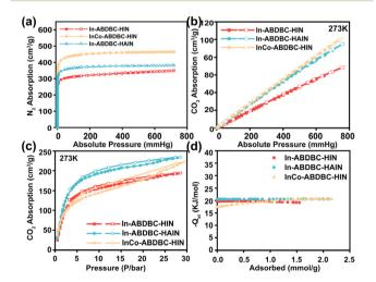
Fig. 3 (a) N<sub>2</sub> adsorption and desorption isotherms at 77 K, (b) lowpressure CO<sub>2</sub> adsorption isotherms at 273 K and (c) high-pressure CO<sub>2</sub> adsorption isotherms at 273 K for In-ABDBC-HIN, InCo-ABDBC-HIN, and In-ABDBC-HAIN. (d) Isosteric heat of adsorption (Qst).
