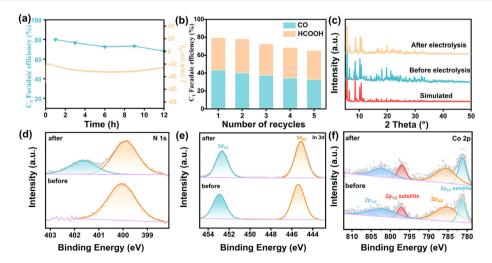
Fig. 5 (a) Long-term durability of InCo-ABDBC-HIN. (b) FE after five times electrolysis at -2.2 V vs. Ag/Ag<sup>+</sup>. (c) Comparison of XRD spectra, (d) N 1s, (e) In 3d and (f) Co 2p XPS of InCo-ABDBC-HIN before and after electrolysis.
