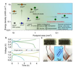
Fig. 4 Comparison of Swiss-roll microbattery performance. (a) Comparison of areal energy density, footprint area, and cycling performance of Swiss-roll microbatteries with previously reported ones. (b) GCD curves of microbatteries connected in series and parallel. (c) Digital photographs of Swiss-roll microbattery powering a digital watch for two min (inset is the encapsulated Swiss-roll microbattery).
