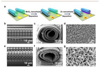
Fig. 2 Manufacture of mesostructured Swiss-roll microelectrodes. (a) Schematic of the Zn-MnO<sub>2</sub> Swiss-roll microbattery fabrication process. Top (b) and side view (c) SEM images of mesostructured Swiss-roll microcathode. (d) Magnified SEM image of the MnO<sub>2</sub> morphology. Top (e) and side (f) view of mesostructured Swiss-roll microanode. (g) Magnified SEM image of the Zn nanosheet morphology
