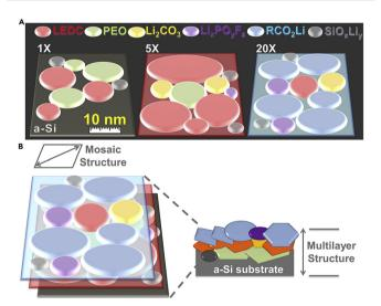
(A) Schematic of the SEI tomography evolution correlated to increasing cycle number probed by tip-enhanced Raman spectroscopy (TERS). (B) Schematic Illustration of the Nanomosaic-Multilayer Hybrid SEI Model on a cycled a-Si surface. Reproduced from ref. 60 with permission from Elsevier, copyright 2019
