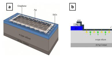
Fig. 2 (a) Schematic of a graphene-on-semiconductor (Si) solar cell. (b) Electron-hole pairs transport across the surface junction. Reproduced from ref. 159, with permission from Elsevier.
