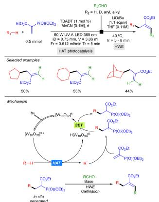
Two-step photocatalytic Michel addition/HWE olefination in flow. Scheme 27
