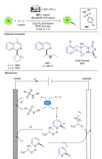
Scheme 43 Electrochemical alkylation of nitrogen heterocycles using an N-alkyl sulfonamide as the HAT reagent.
