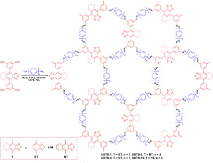
Fig. 8 Schematic diagram for synthesizing USBT-7 to USTB-10.81
