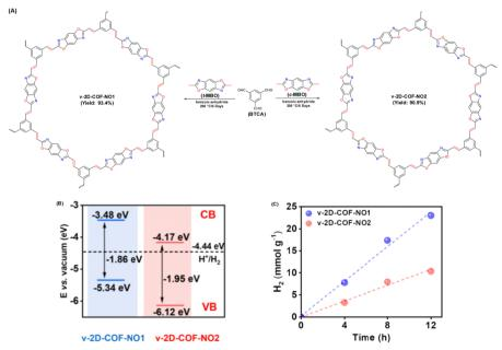
Fig. 12 (A) Schematic illustration for establishing v-2D-COF-NO1 and v-2D-COF-NO2. (B) Energy band position of v-2D-COFNO1 and v-2D-COF-NO1 NO2. (C) Time course of photocatalytic H<sub>2</sub> production activity for v-2D-COFNO1 and v-2D-COF-NO2. Reproduced with permission, copyright, 2022, American Chemical Society.94
