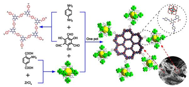
Fig. 19 Schematic illustration for designing an NH<sub>2</sub>-UiO-66/TpPa-1-COF hybrid material. Adapted with permission, copyright, 2018, Wiley-VCH. 124
