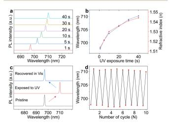
Fig. 4 (a) Time-dependent lasing spectra of the BIPS@PMMA filmcovered Ag nanoparticle array on exposure to UV light. (b) Plots of the lasing wavelength and refractive index of the BIPS@PMMA film-covered  $\mbox{\sc Ag}$ nanoparticle array versus time of exposure to UV light. (c) Lasing spectra of the BIPS@PMMA film-covered Ag nanoparticle array under alternate irradiation with UV and Vis light. (d) Plot of the lasing wavelength versus switching cycles.
