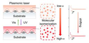
Scheme 1 Schematic illustration for wavelength-tunable plasmonic lasers based on photoisomerization-activated change of refractive index.
