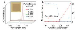
Fig. 3 (a) PL spectra of the BIPS@PMMA film-covered Ag nanoparticle array at different pump fluences. Inset: Bright-field microscopy image of the fabricated device. Scale bar is 50 µm. (b) Emission intensity (red) and FWHM (blue) as a function of pump fluence.
