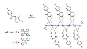
Scheme 1 Formation of coordination polymers of Ag<sup>+</sup> with thiol ligand 1 and its control compound 2. Dashed lines through the backbone represent Ag+...Ag+ interactions.16
