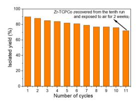
Fig. 2 Recyclability of the photocatalyst Zr-TCPCo.
