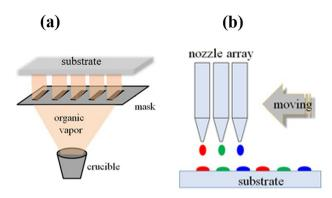
Fig. 1 Schematic diagrams of thin-film fabrication: (a) vacuum evaporation and (b) inkjet printing
