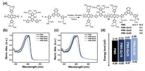
Fig. 1 (a) Synthetic routes and chemical structures of the alternating copolymer and random terpolymers. UV-Vis absorption spectra of the corresponding polymers in (b) dilute solution and (c) thin films. (d) Energy level diagrams of the corresponding polymers.
