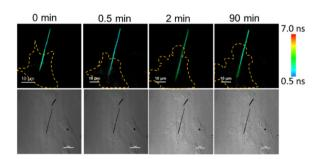
Fig. 4 The FL images of the NWFLT incubated with a single cell after adding 125  $\mu\text{M}$  cisplatin for various times as shown in the top row. The DIC images of the NWFLT and the single cell at various times are shown in the bottom row. The cells are noted by the yellow dotted line, and the scale bars of the DIC images are 20 µm.
