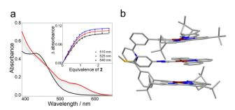
Fig. 2 (a) UV/Vis absorbance changes of  $\bf 1$  at 298 K (c = 0.05 mM in CH<sub>3</sub>CN) upon the progressive addition of 2. Inset: intensity changes in UV/ Vis absorbance at 510 nm, 525 nm, and 540 nm. The solid lines were obtained via a Matlab-based global analysis program. (b) Optimized structure of the host–guest complex  $1 \supset 2$  on the basis of DFT calculations.
