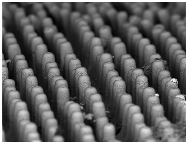
Fig. 27 SEM photomicrograph of pillar array of sintered YSZ overprinted with sintered LSM.
